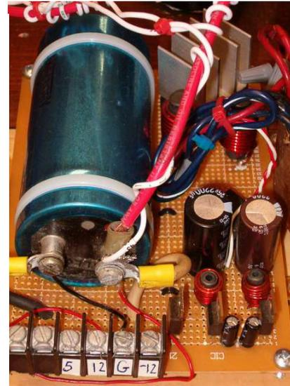
Below is the complete Plasma Speaker assembly in operation. Note the use of two ignition coils allows a long hot spark of modulated plasma to be created between the high voltage terminals. This is not found in other Plasma Speaker designs shown in this paper which discharge from a single point into the surrounding air.
